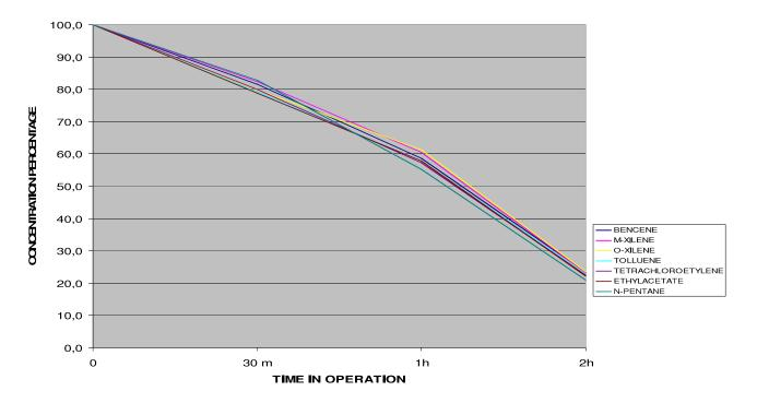
It can be seen that after the eCo3 equipment has been working for 2 hours the concentration of Volatile Organic Compounds analysed is reduced to an average of 22.3% compared to the initial maximum values. When the same measurement is taken without the air treatment equipment working, the average reduction values obtained with respect to the maximum value was 53.1%.
