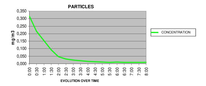
As can be seen in the graph, there was a reduction in the concentration of particles in the first two hours during which the equipment was functioning and thereafter the concentration readings remained very low.
